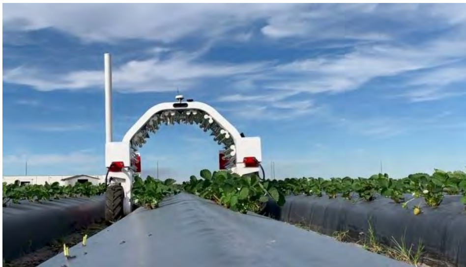
Figure 5 (Entraid). Here at work on strawberries, the Thorvald robot should soon arrive in a vine configuration. It applies UV at night to fight against powdery mildew and downy mildew. You have to use it quite often, hence the idea of a robot.
