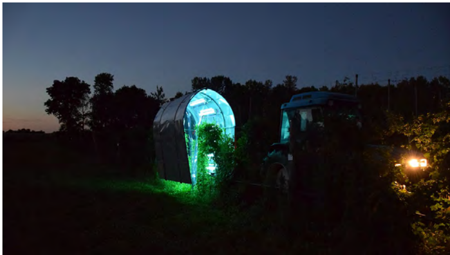
Figure 3 (Provided). The Light and Plant Health project team, led by Cornell AgriTech's David Gadoury, has developed inexpensive, efficient lighting and delivery systems, such as low-tech tractor attachments, to treat plants with UV light.
